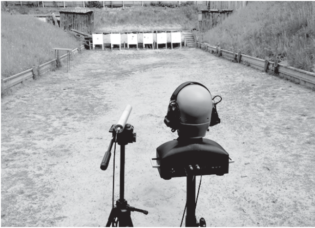
In the foreground: left – a GRAS 67SB transducer used for measuring the properties of acoustic impulses, right – a GRAS 45CB acoustic test fixture to measure the acoustic properties of hearing protectors, with level-dependent earmuffs (test object). The impulse noise is generated by discharging the firearm operated by a shooter (not shown in the photograph).
