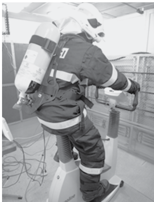
Photo 2. Fire fighter in a standard rescue suit with breathing apparatus on a bicycle ergometer in the model work (load value: 100 W) inside the climatic chamber
