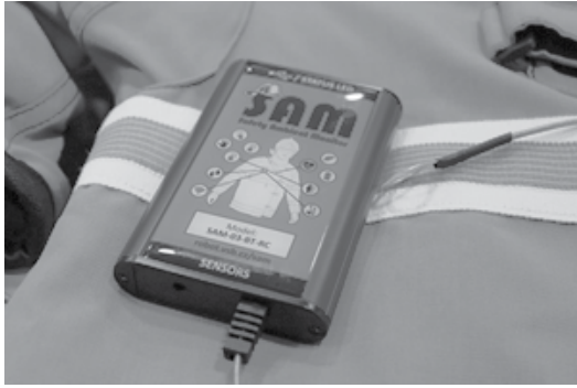
Photo 1. Safety Ambient Monitor (SAM) – the tested device measuring thermal exposure of fire fighters and members of rescue teams, and signaling the strain of rescuers and the indicators of physiological response of the body
